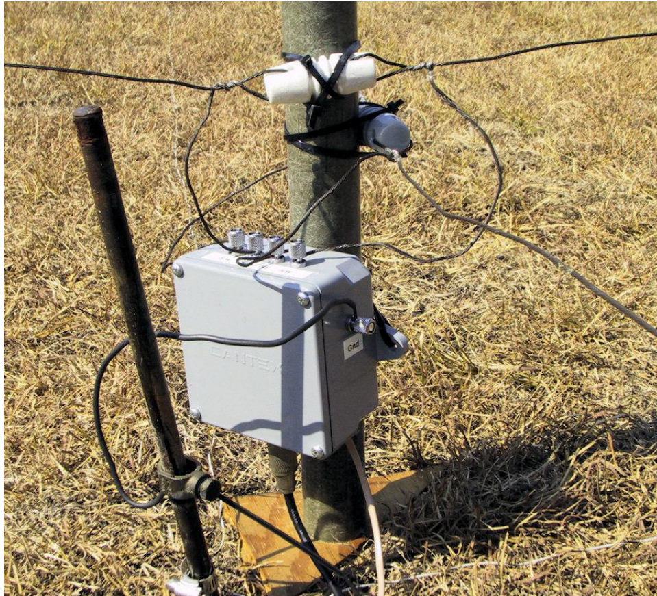
Figure 3: Attachment of the bottom of the loops.
